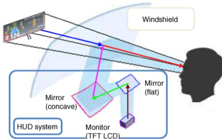
\* Video on the monitor is reflected with 2 mirrors and virtual image is displayed on the windshield.
