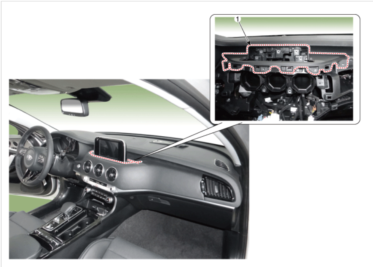
1. Monitor fascia panel
