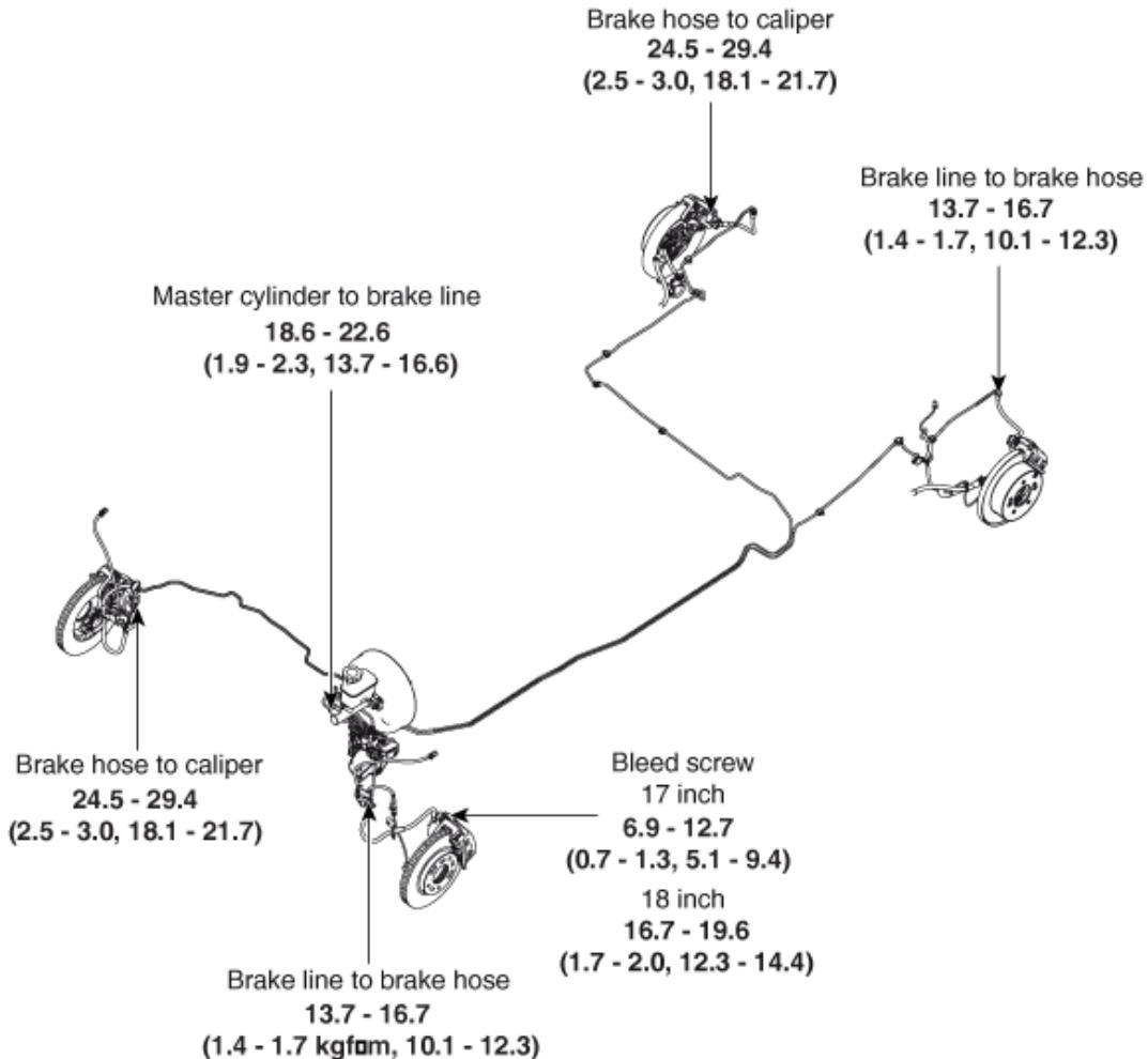
**Tightening torque : N·m (kgf·m, lb·ft)**
