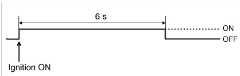
3. When the ignition is switched ON during variant coding (EOL) mode, the airbag warning lamp will illuminate and blink at intervals of 1 second until the coding is completed.
