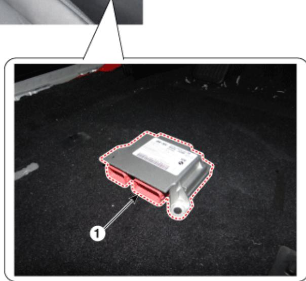
1. Supplemental Restraint System Control Module (SRSCM)
