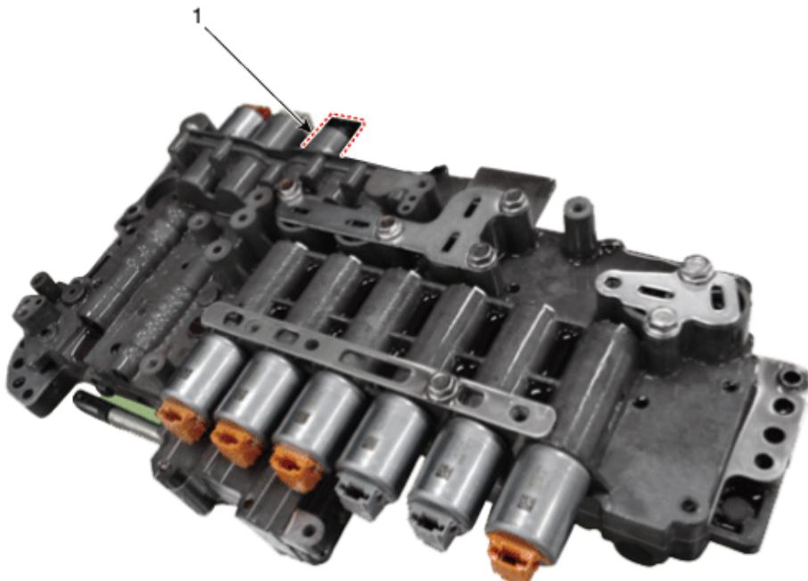
1. SS-A solenoid valve (ON/OFF)
