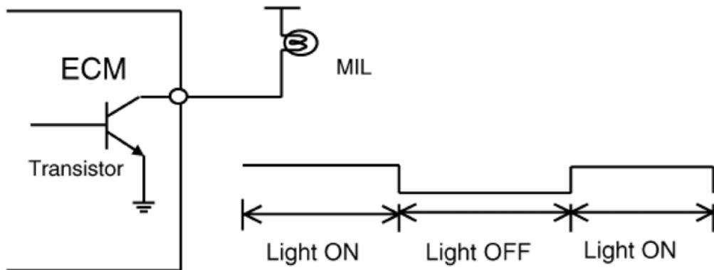
The Malfunction Indicator Lamp (MIL) is connected between ECM or PCM-terminal Malfunction Indicator Lamp and battery supply (open collector amplifier).
