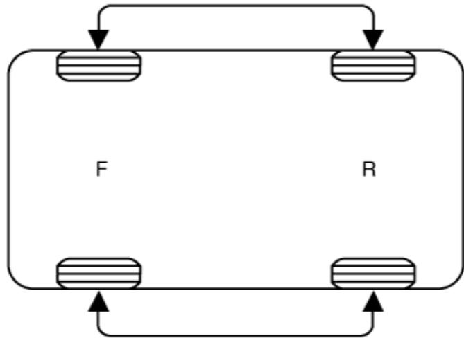
3. If the steering continues to pull to one side, rotate the front right and left tires again, and perform a road test.
