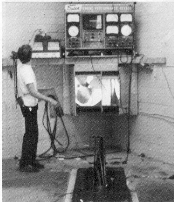
Below left: Sun infrared exhaust analyzer forms the basis for the first home-built motorcycle dyno inside Dobeck's Wisconsin shop, circa 1980. Below right: Dobeck demonstrating the Dynojet 100 to motorcycle enthusiasts in Macao, China—he's traveled the world promoting his products and the notion of honest tuning.
