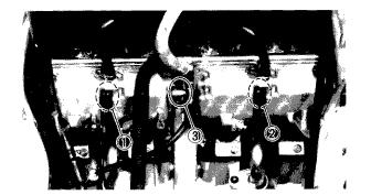
Racing the engine for less than a second, two or three times, and check the synchronization again.
